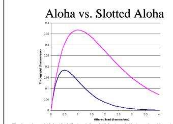
The throughput of Aloha (dark line) and slotted Aloha (purple line) are plotted here. As the load on the network increase, the throughput increases at first. As the network gets busier, the throughput starts to decline until very little data is successfully received when the network is very busy.
